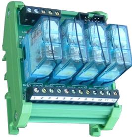
Passive relay interface module that receives commands from electronic equipment such as PLCs, industrial PCs, control modules, etc. and controls inductive and resistive loads of small power such as solenoid valves, contactors, small servomotors, lamps, resistors, etc. This type of module has a series of screw terminals that makes it universal and a multi-pin flat connector for quick connections.
